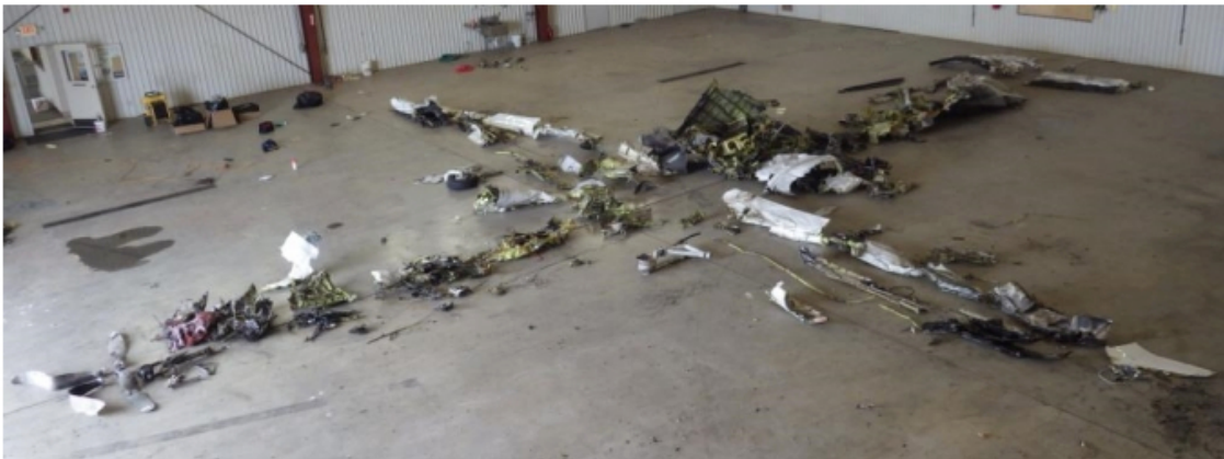
Figure 5 – Wreckage organized in hangar
